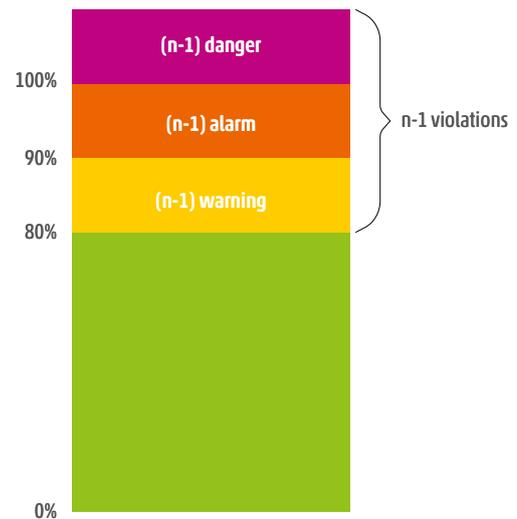
Figure 1.7: Example for alarm thresholds in n-1 calculation
