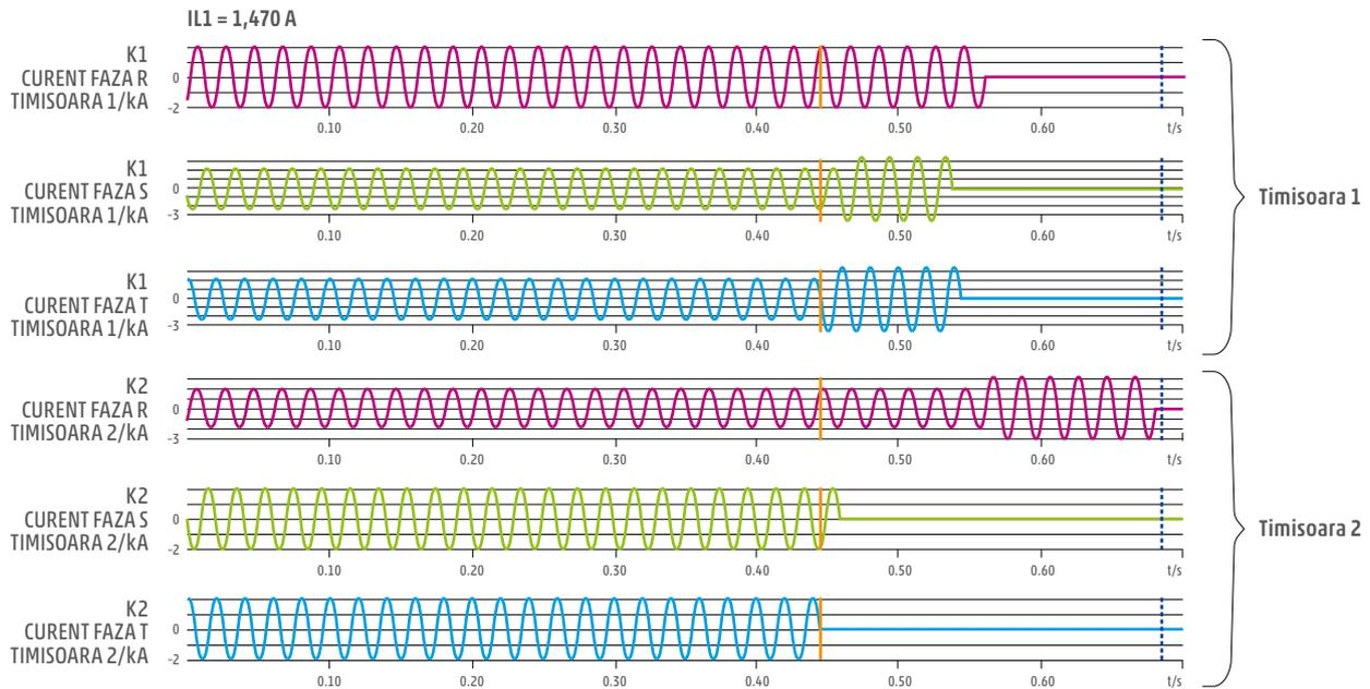
Figure 2.7: Resita-Timisoara protection device oscillo recordings (instantaneous values)
