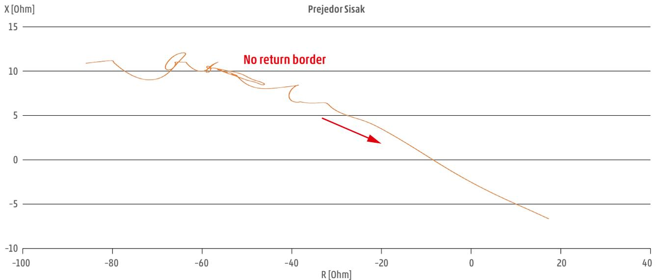
Figure 2.14: Simulation of distance protection activation X-R Diagram
