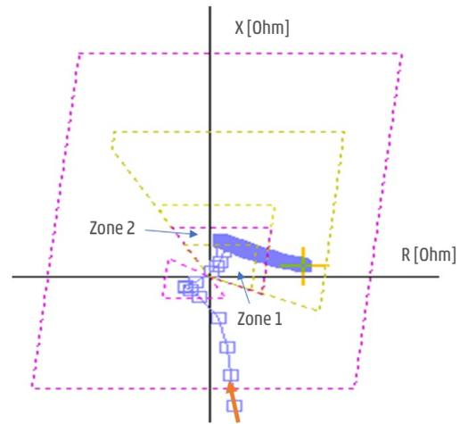
Figure 2.9: Mintia - Sibiu protection device X R diagram (real recording)
