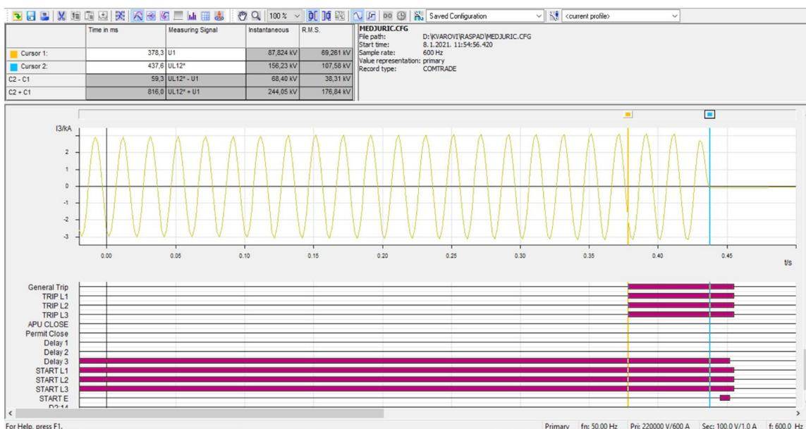
Figure 2.8: Meduric – Prijedor protection device recording (oscillo instantaneous values and internal signals event recording)
